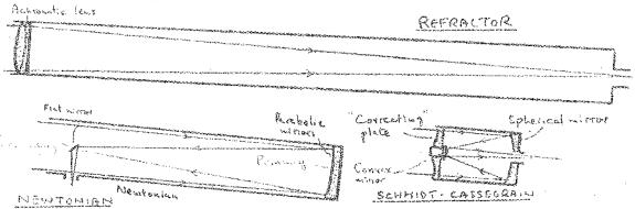
While giant refractors were built in Victorian times, almost all modern large professional adescopes are of Cassegram design, while the Schmidt telescope serves as a wide-field camera with fast f-ratio.
